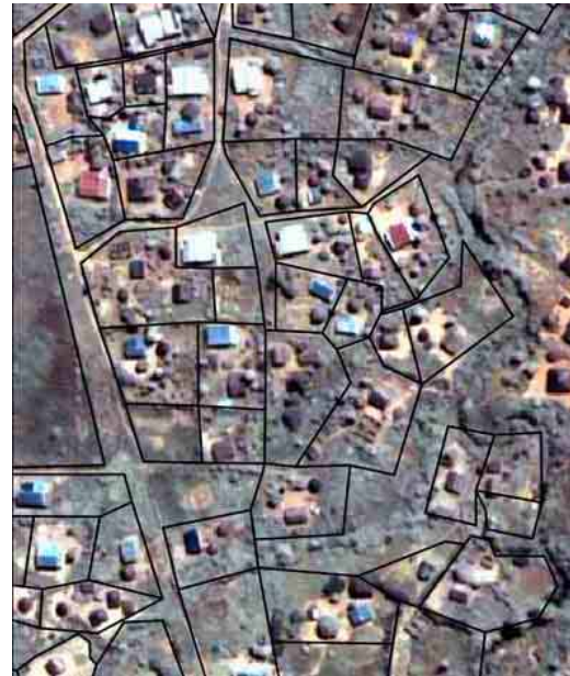
Figure 23. Manica. Neighbourhood Josina Machel. Satellite Image (March, 2003) Quick Bird Sub-meter (0.6m) PSM (true color) with aprox. Restitution and terrains lots delimitation (talhões).
